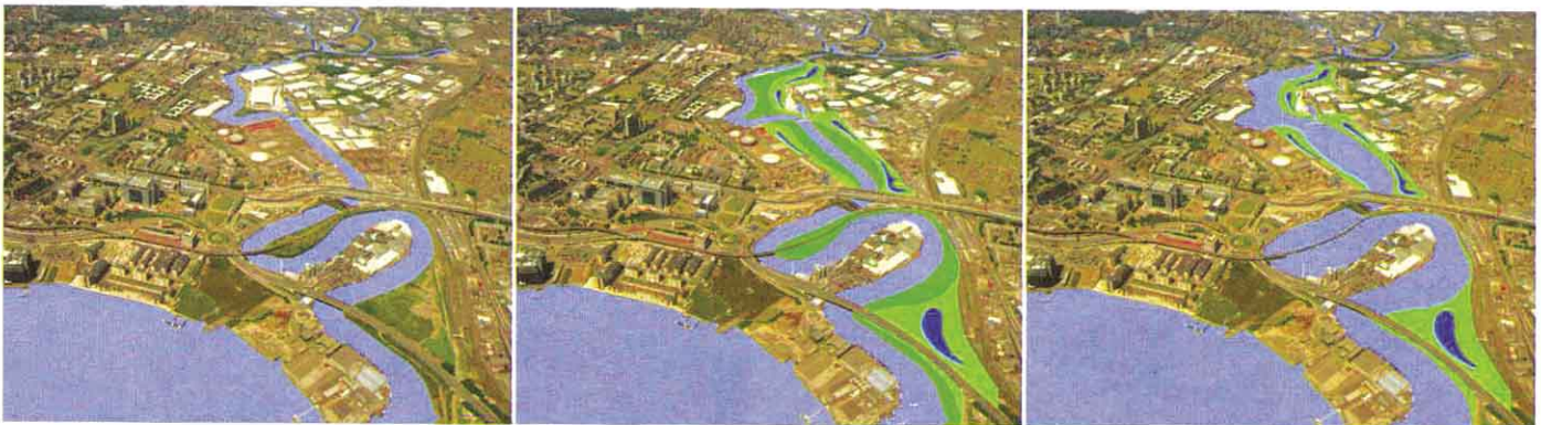
The Lower Lea Valley will become an area of major urban regeneration, regardless of whether London's bid for the 2012 Olympics is successful. Part of the Farrell/Lovejoy proposals for the site included the removal of some flood-defence walls which would allow the river to expand into flood-alleviation buffer zones. These areas along the riparian corridor would also accommodate stormwater wetlands to attenuate runoff. (Image courtesy Lovejoy)
